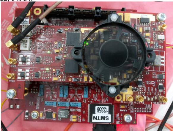
Fig.10. FPGA carrier board used for verification of degarbling algorithm
