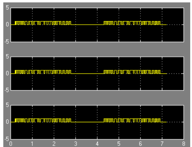
Fig.9b. simulation result for degarbling detection of individual data pulse train
