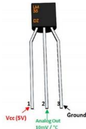
Fig. 3. LM35 Temperature Sensor [18].
