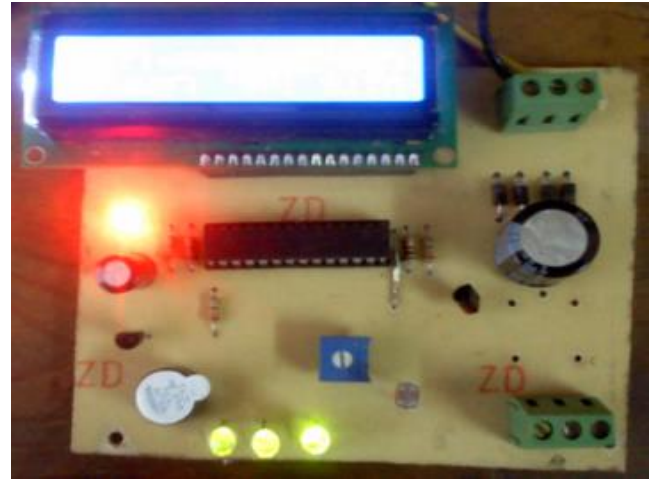
Fig. 19. The practical result when the LEDs are ON-Yellow, during low light intensity, according to step 3 in the system flowchart.
