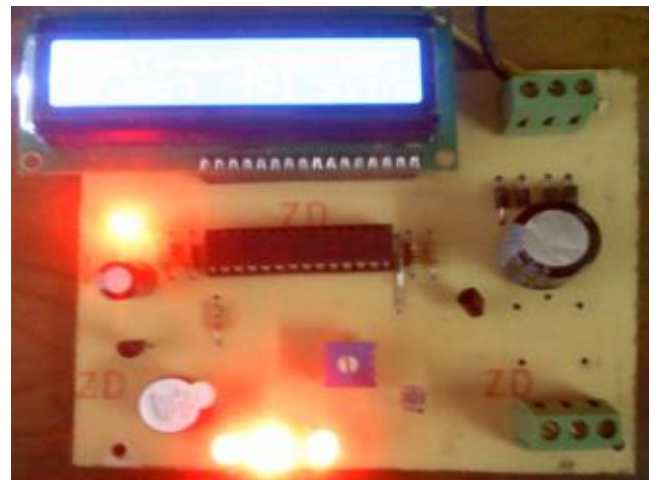
Fig. 20. The practical result when the LEDs are ON-Red, during low light intensity, according to step 5 in the system flowchart.
