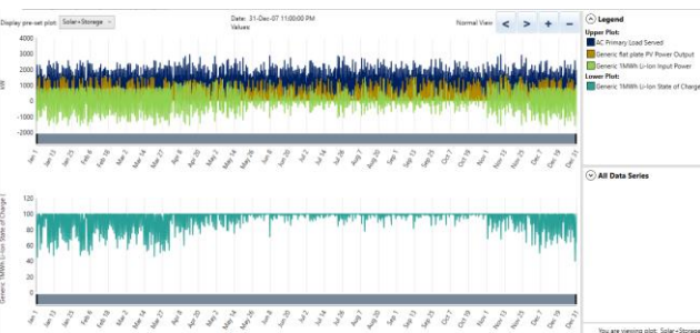
Fig. 15: Hourly plot of solar PV system and energy storage output illustrating the performance of the solar PV system and ESS
