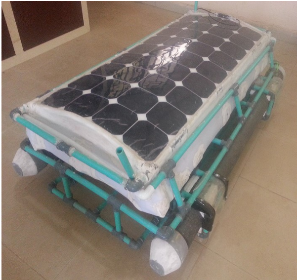
Fig. 23. The Process of the Skeletal Frame made up of PVC Pipe Enclosed with Fiber-reinforced Plastics for WMUSV
