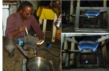
Fig. 6. During water boiling test
