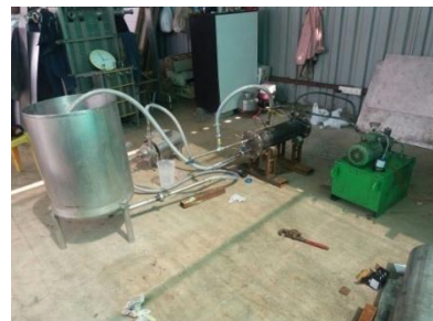
Fig.4.7:- Shell & Tube Heat Exchanger during trial
