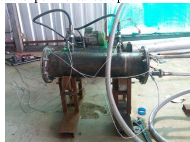
Fig.4.6:- Shell & Tube Heat Exchanger before Trial
