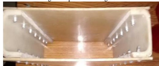
Fig.8. Front View of Wing Box
