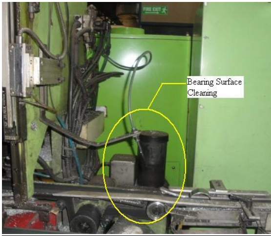
Fig 12 : Bearing Surface Cleaning
