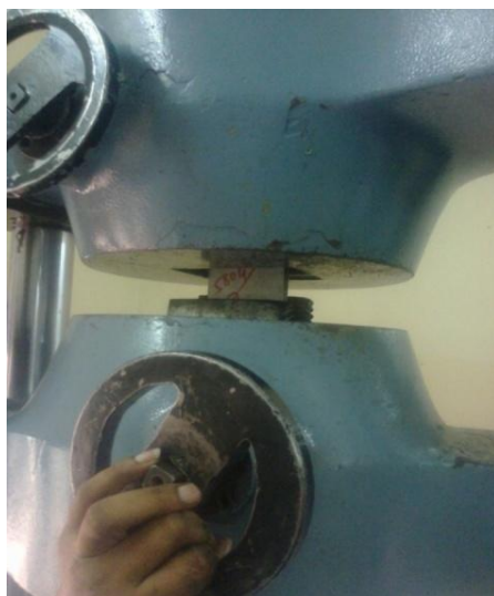
Fig 4.2 Tensile test of the specimen by using UTM
