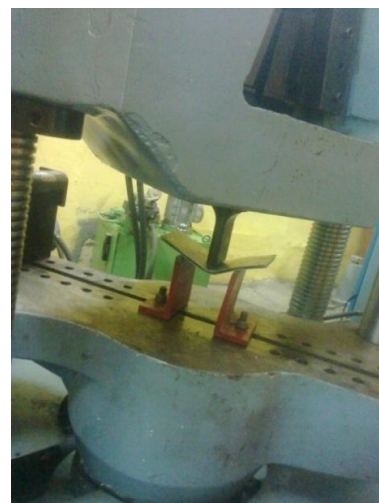
Fig. 5.1 Experimental set-up of bending test
