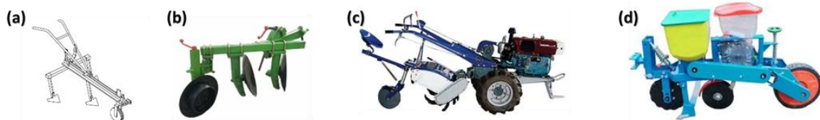
Fig. 2: Option of soil engaging components: Animal draft cultivator (a) [1]; Disc plough (b); Rotovator (c); Precision planter (d).
