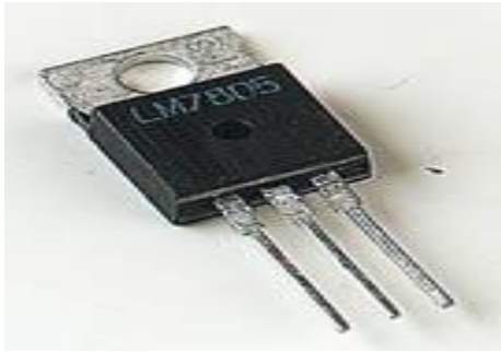
Fig.3.2.2.2 Voltage regulator LM7805 [11]
