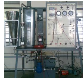
Figure 1: Experimental Setup of a cylindrical Tank level system
