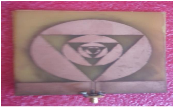
Figure 3. Fabricated UWB crown fractal antenna
