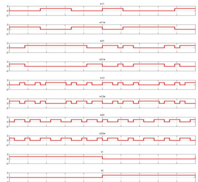
Fig.7. Switching pulses for 17-Level Converter
