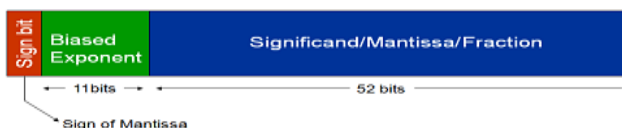
Fig 1: IEEE-754 Double Precision Floating Point Number Format
