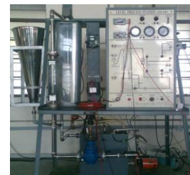
Figure 1: Experimental Setup of a Conical Tank level system
