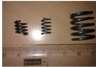
Fig. 3 SMA springs used for verification of the model
