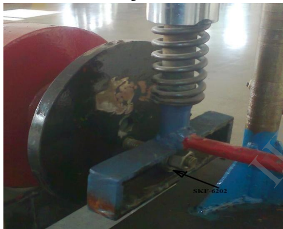
Fig.2 SKF 6202 bearing connected with disc protrusion
