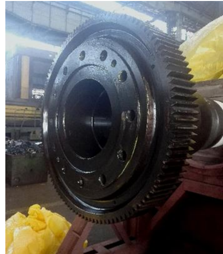
Fig. 7, Gear shrunk on over a turbine coupling
