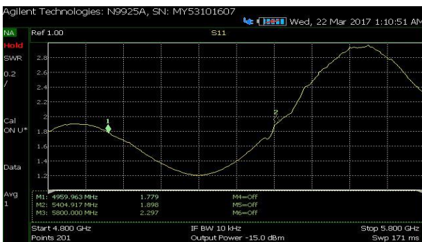
Figure 8. Measured SWR by Network Analyzer at 5.4GHz
