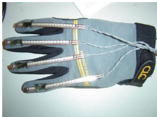
Fig.7 Glove with flex Sensors
