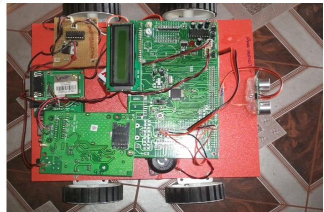
Fig-2: Hardware Implementation of accidental vehicle using GPS and MEMS accelerometer
