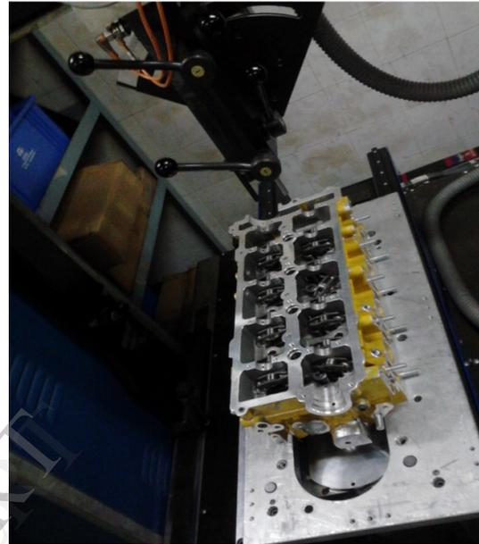
Figure 2. Experimental set up for flow coefficient measurement
