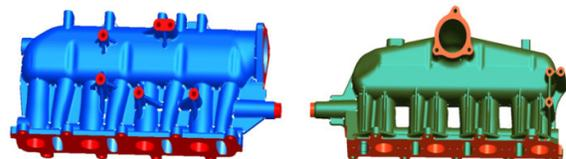
**Figure 8.** Intake Manifold CAD model by using Pro/Engineer
