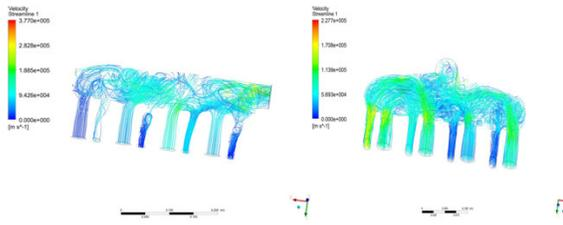
Figure 9. Intake Manifold streamline CFD model
