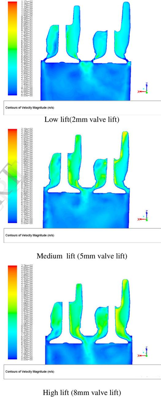
Figure 16. Velocity contours
