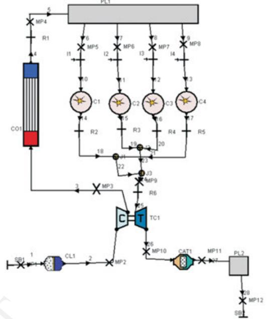
Figure 12. One dimensional analysis model for engine performance characteristic by using AVL boost software
