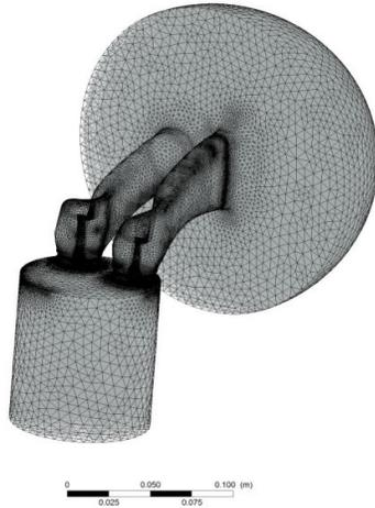
Figure 6. Mesh creation of intake port
