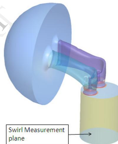
**Figure 5.** Intake port computational model
