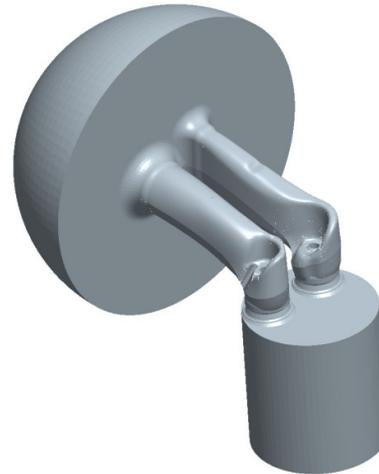
**Figure 4.** 3D cad model of intake port
