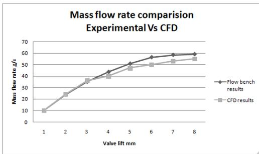
Figure 10. Mass flow rate comparison graph
