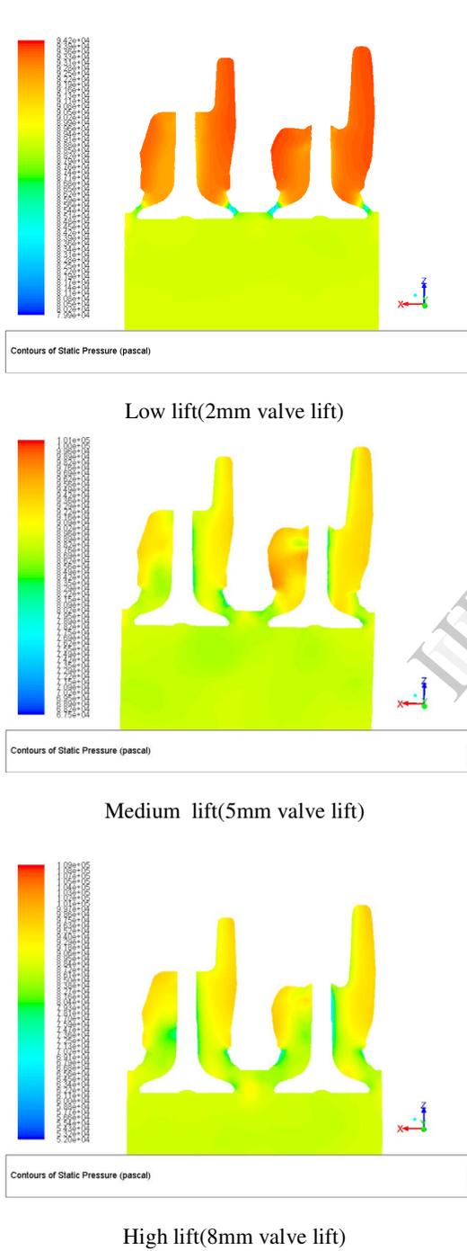
Figure 15. Static pressure contours
