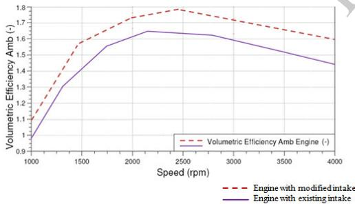
Figure 11. Volumetric efficiency comparison graph
