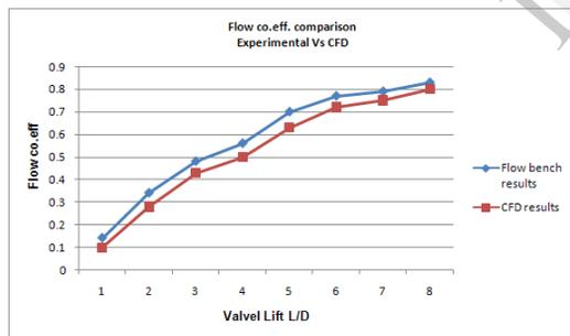
Figure 17. Flow co-efficient comparison graph
