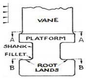
The blade forces, centrifugal forces (radial) and into axial and circumferential bending forces. For the consideration of stiffness effects of both the rotor (drum or disc) and the blade root, the reduction of the bending force into its axial and circumferential component is required.
