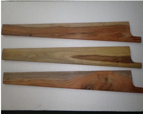
Fig 8 The Structure of fabricated timber blade
