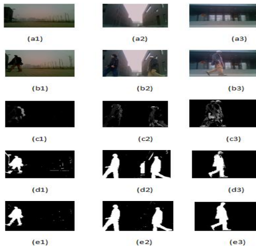
Fig. 7 Results from different algorithm, ((a1), (a2), and (a3)) are background images, ((b1), (b2), and (b3)) are feed video inputs from camera, (c1), (c2), and (c3) are detection results from frame differencing, ((d1), (d2) and (d3)) are detection results from background subtraction, ((e1), (e2) and (e3)) are detection results from proposed system (hybrid adaptive scheme)
