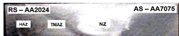
Figure 4. Typical cross section of the weld (600rpm, 30mm/min, 2.5kN, TT tool) shows the NZ, TMAZ and HAZ.
