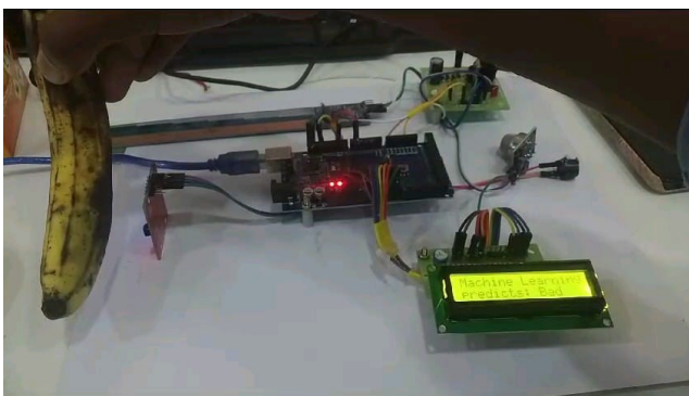
Fig 6: ML predicts bad fruit in LCD and Buzzer alerts
