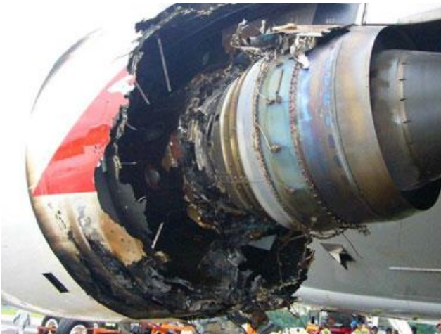
Fig. 2 A Rolls Royce Trent 972 intermediate pressure turbine disk burst accident which occurred near Singapore (Hradecky, 2010)
