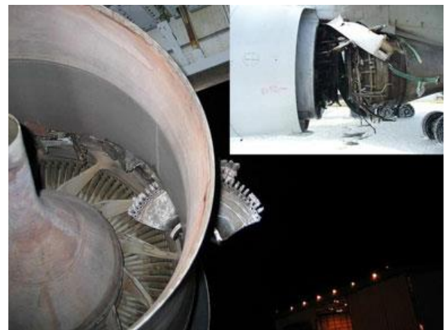
Fig. 1 A CF6-80A2 high pressure turbine disk burst accident which occurred at Los Angeles International Airport (Aviation Safety Network, 2006).
