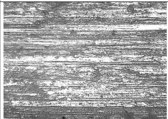
Wear track of En 31 steel disc – Micro Photo graph
