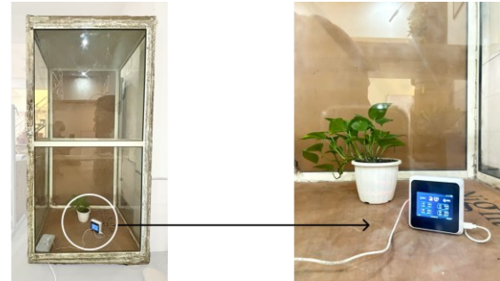
Fig. 2 Experimental set up of Epipremnum aureum in test chamber for testing PM 2.5 and TVOCs
