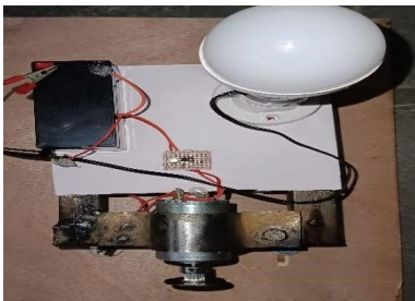
Figure 1: Load, generator & battery systems
