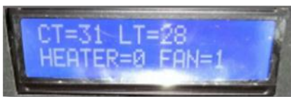
Fig 11: LCD result display for third experiment
