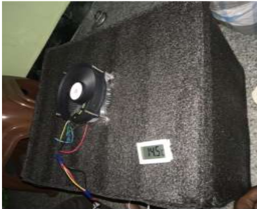
Fig 3.2 TEC-12705 refrigeration unit
