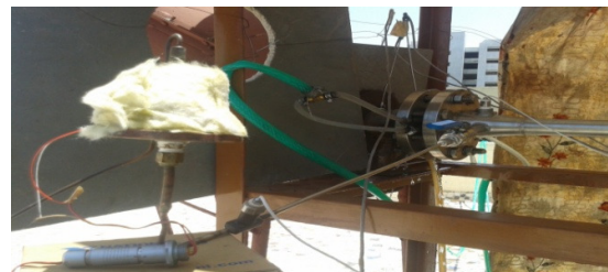
Fig 4.1: Standing wave engine driven pulse tube cryocooler.
