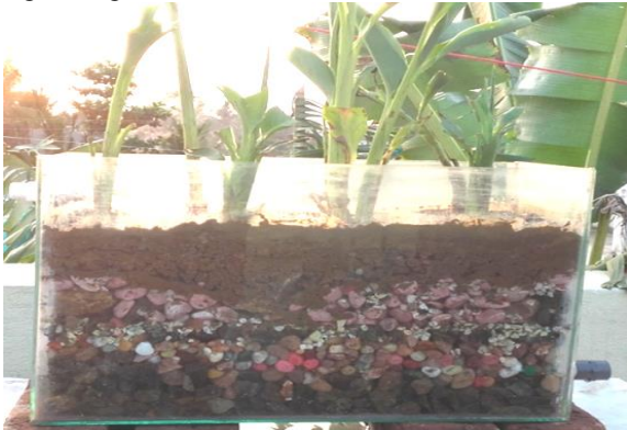
Fig2. Typical section of the biofilter tank
