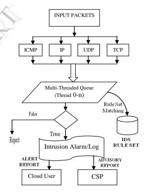
Fig.2 Flow Chart for Double Guard
