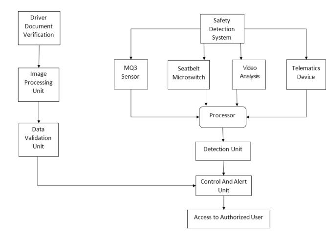
When the driver submits the document, the documents are verified and validated by using an image processing unit after validation the document will be uploaded. The safety precaution system has four sensors and if any safety violation has been detected it will send a notification to the admin.
