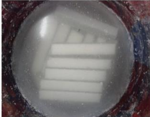
Fig.5: Submersion of mortar bar into lime water bath.
