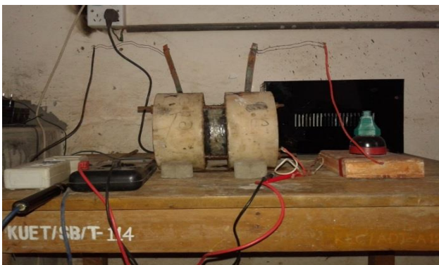
Fig.2: Experimental setup for penetrability test.
