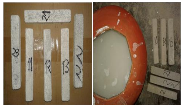
Fig.4: Preparation and submersion of sample into lime water bath.
