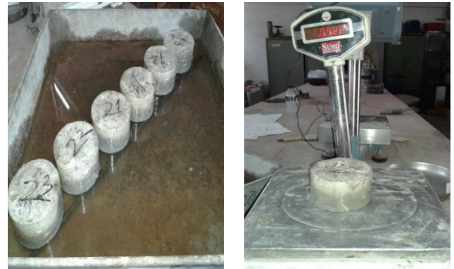
Fig.3: Experimental setup for water sorptivity test.
