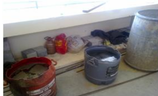
Fig. 4. Cubes immersed in acid solution 7 days, 30 days and 70 days.
