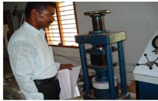
Fig. 11. Compressive strength test on cube
