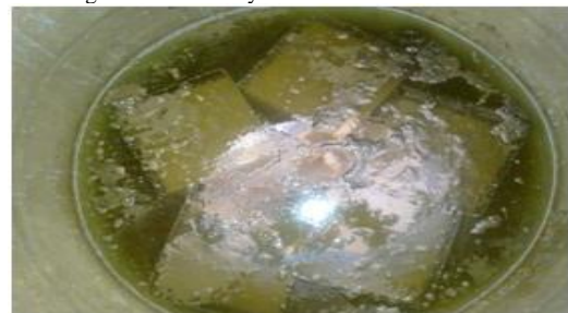
Fig. 3. Cubes 70 days immersed in acid solution
