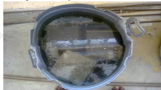
Fig. 2. Cubes 30 days immersed in acid solution
