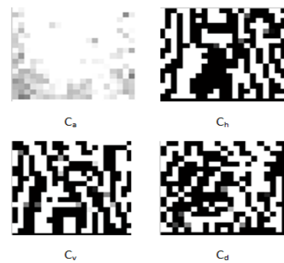
“Figure 5. 3 rd level DWT a) Approximate coefficients b) Horizontal coefficients c) Vertical coefficient d) Diagonal coefficient”
