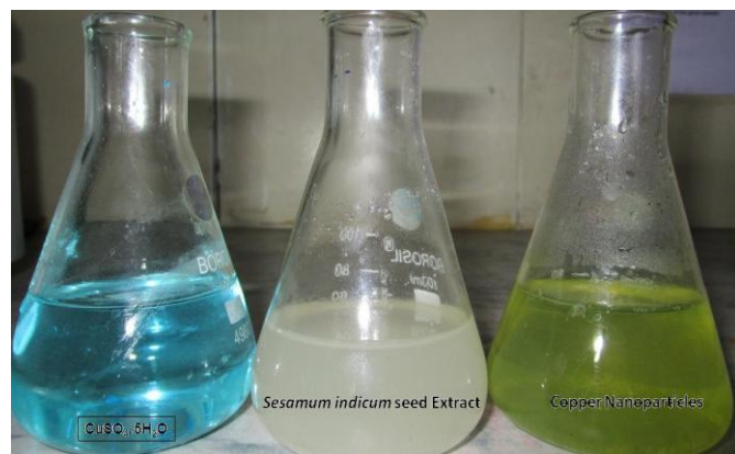
Figure-2: Change in colour of Sesamum indicum seeds extract during copper nanoparticles synthesis
