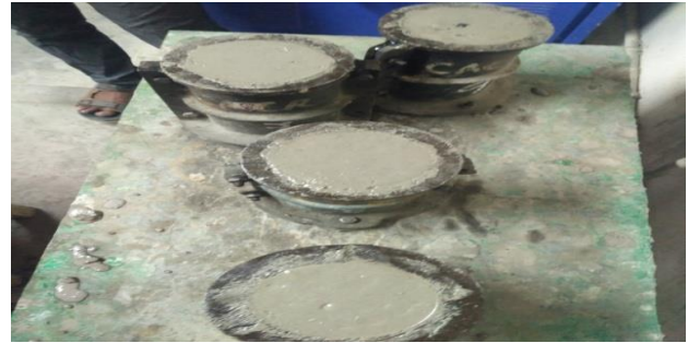
Fig 2: casting of cylinder
