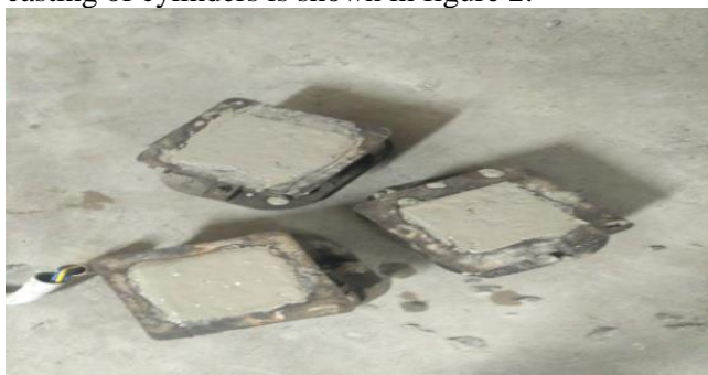
Fig 1: Casting of cubes
