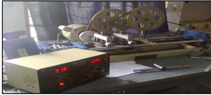
Figure 3. Testing Equipment Electronic Tensometer
