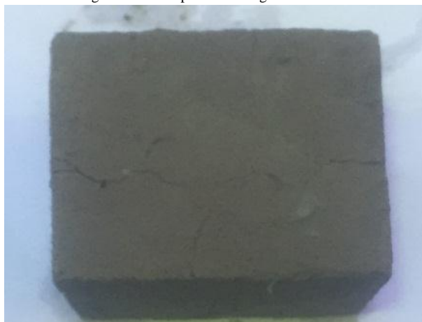
Figure 5: S3 sample after firing at 900°C and sudden wet cooling.
