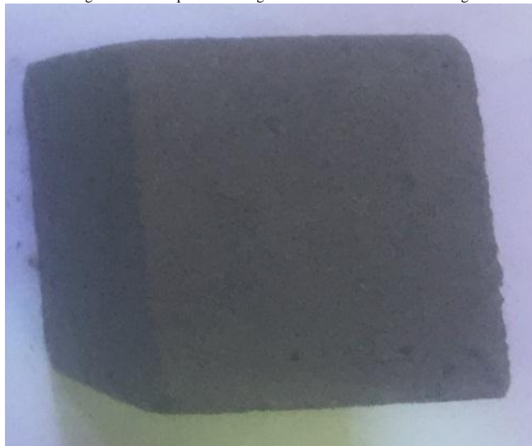
Figure 7: R2 sample after firing at 900°C and sudden wet cooling.
