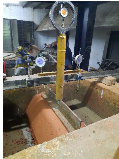
Fig 3. Arrangement for measuring Load and Settlement
