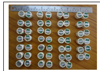
Fig. 5. Specimens for measuring weld pool geometry
