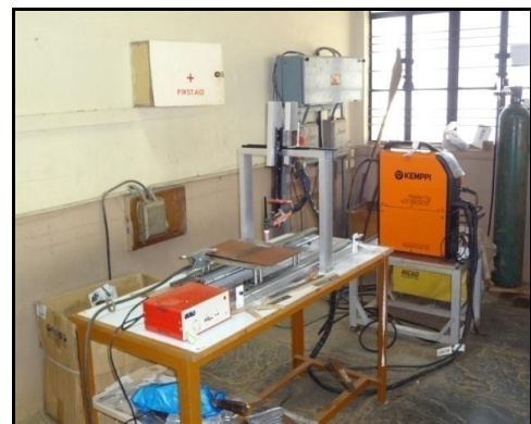
Fig. 2: Experimental set up for GTAW.
