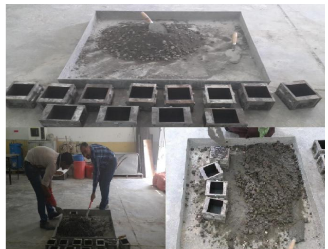
Figure (1) Concrete casting and molding
