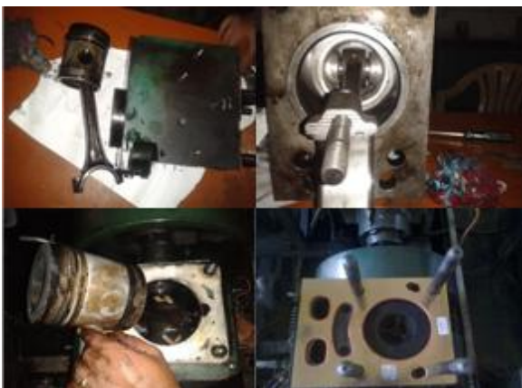
Fig 2 : Arrangement of modified piston inside the engine cylinder
