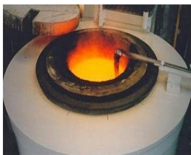
Figure 2- Salt bath furnace used in heat treatment with molten salt as the heating medium.
