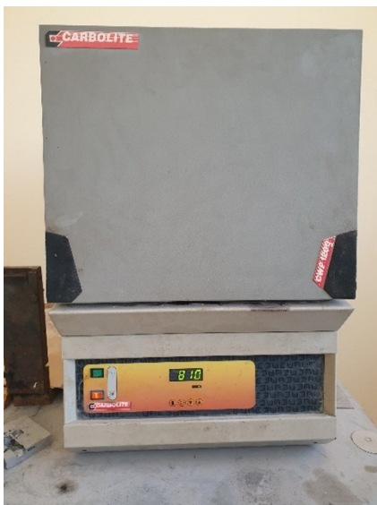
Figure 1- Box furnace used in heat treatment with the austenitization temperature set to 810 0 C.
